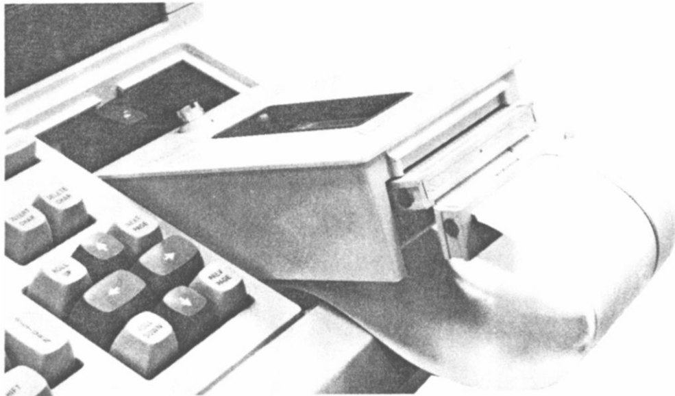
Figure 5-1. Model 64516A PROM Programmer Module Being Installed
